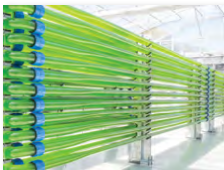
▲ Figure 7.3: Tubular fence photobioreactor with 10-m glass tubes
